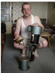
Cavity with tube - Long 75 cm, weight 25kg
