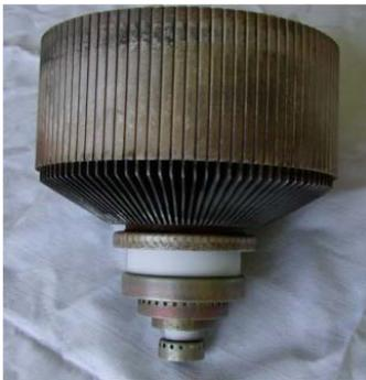
The TH 313 is a forced air-cooled ceramic metal tetrode, of coaxial structure. It can be use as a C.W. oscillator, or a grounded grid R.F. power amplifier at frequencies up tu 1,3 GHz. The anode can dissipate 7,5 kW.
