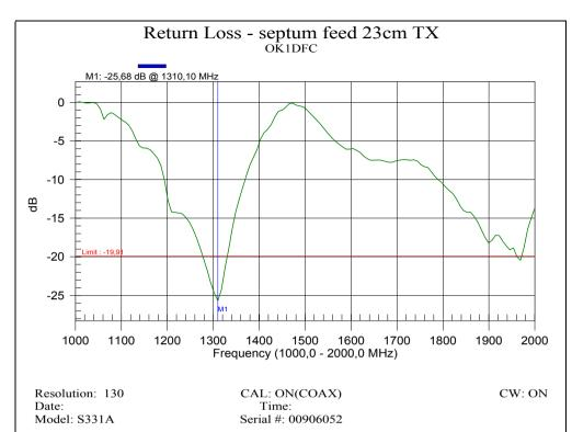
Minimum SWR in free space is -26 dB. In the dish is possible setup -36 - -40 dB without problem. You can see the diagram how is looking feed inside dish on my web.
