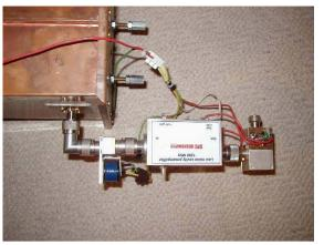
Picture how is looking assembling with isolation relay and preamplifier. This preamplifier is DFC microwave cavity system with 0,4dB N/F. 3.th place in preamplifiers contest trough **EME** 2002 conference Praha
