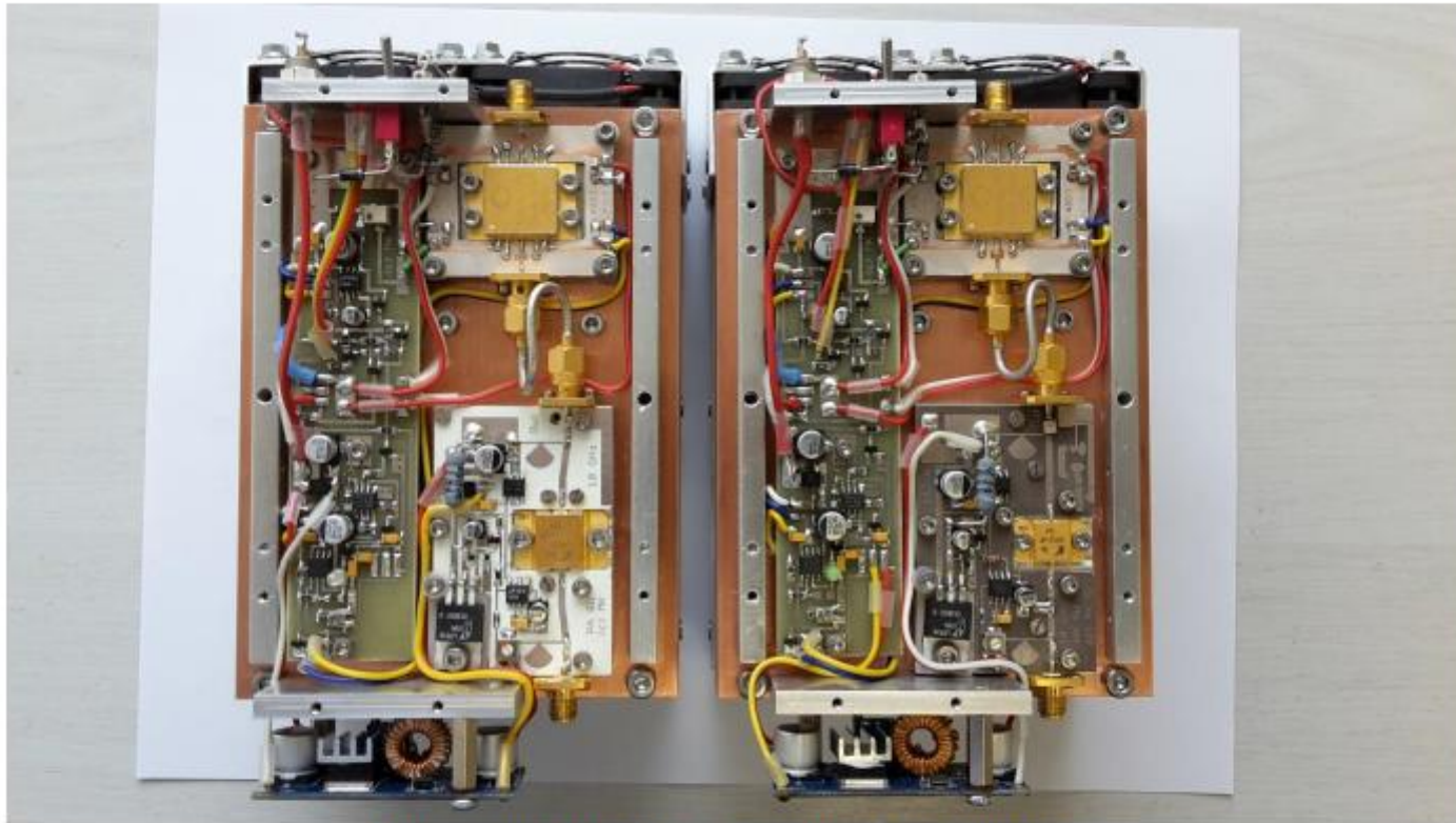
Figure 1. Two 10 GHz power amplifiers with TGA2312FL
